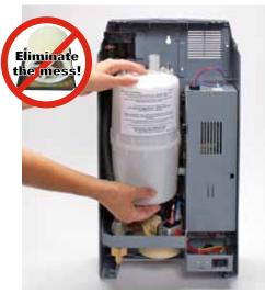
All scale and mineral sediment is deposited into the cylinders which are easily changed and discarded. Cylinder replacement requires no special tools and can be done in a few minutes. A light on the unit indicates when the cylinder needs replacement.
